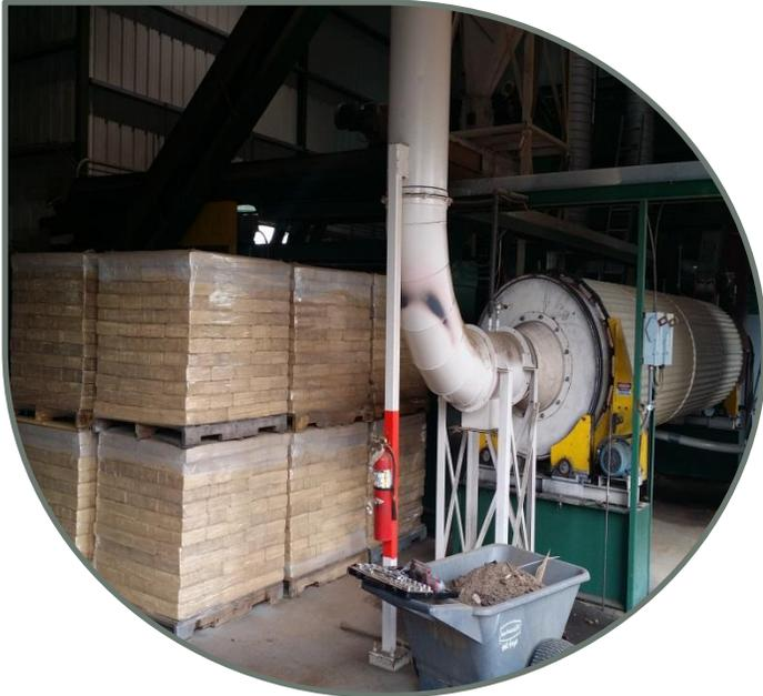
Above: Viking biobrick machine uses wood biomass byproducts from old growth harvests to produce fuel. Lessons from these approaches to biomass utilization can be applied to young growth in the future.
